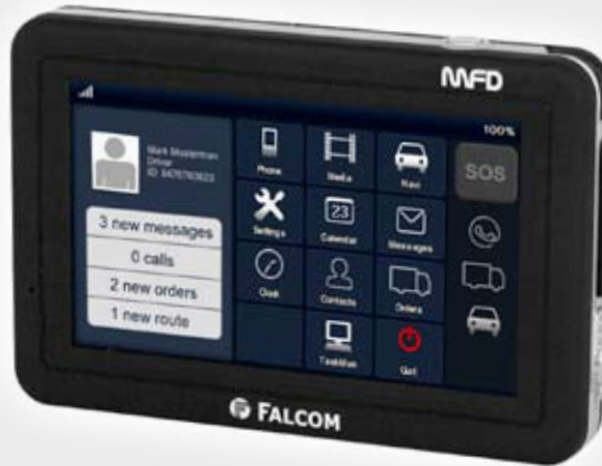
MFD1 - Falcom AVL device controller and stand alone navigation unit*
